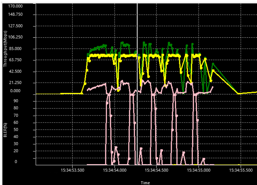
Figure 5.40: Example of application layer throughput and BLER fluctuations during the test cases measured using the QXDM application.
