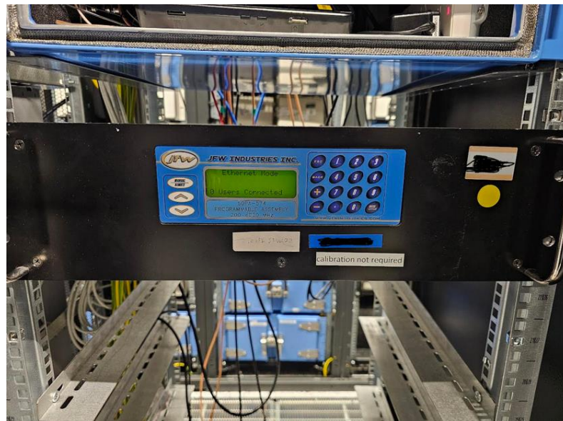
Figure A4.3: Programmable attenuator JWF Industries model 50PA-574.
